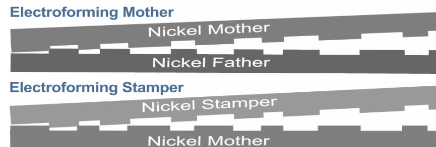
Figure 10 Electroforming Mother & Stamper
