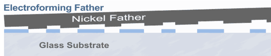
Figure 9 Electroforming Father from Glass Master
